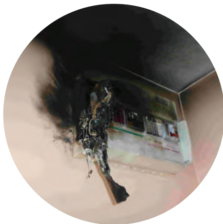
Result of DIY work by a home owner where a 10.5 kW electric shower was connected to a 45 A circuit-breaker using 2.5 mm 2 cable. (Photo courtesy of British Gas)
